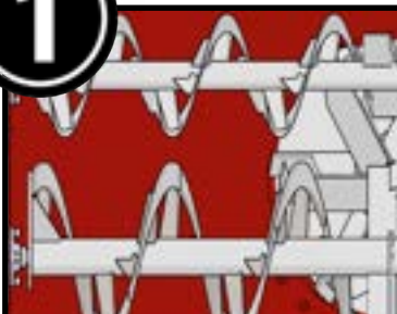
Dual Augers with High Tensile Ribbon Flighting
