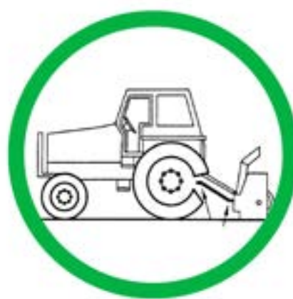
Acceptable Equal Angles at PTO Joints
