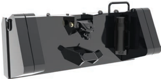
Ballasted to add 1400 lbs to increase drilling down pressure.
