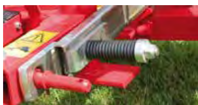
Spring loaded breakaway
