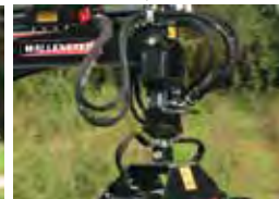
360 Hydraulic Rotator (R & PR models)
