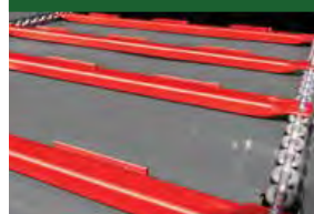
Heavy duty bed chain resulting in less tensioning adjustments
