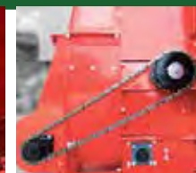
Chain drive to crossbeaters ensure a reliable transmission
