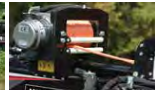
9,000 Warn Winch & 100' Synthetic Rope (RP Models)
