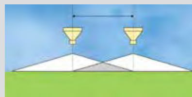
Cone shape pattern provides total overlap
