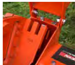
Twig Breaker Discharge paddle passes around the twig breaker and breaks material into smaller pieces.
