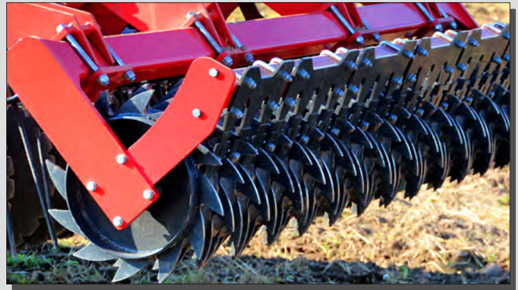
PACKER ROLLER: A heavier more aggressive roller for crushing clods and a firm seedbed.
