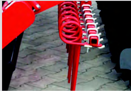
Coil tine spring levelers between discs and rollers.
