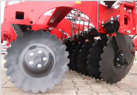
Two rows of individually mounted 22" diameter discs.
