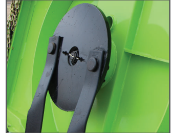
Heavy duty 3/4" thick blade disc with 4" blades and pentagon blade bolts
