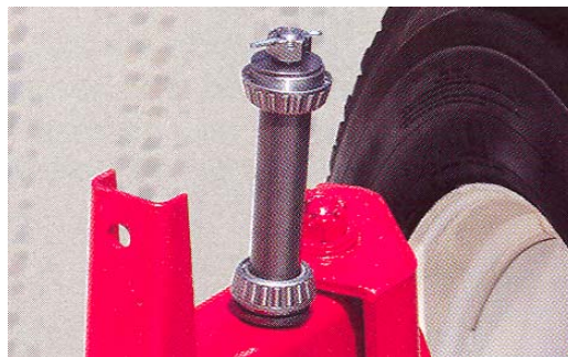
Kingpin Bearings – Standard on all wagons
