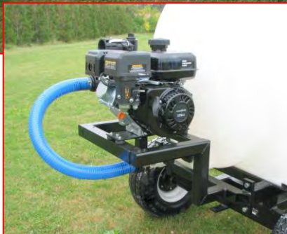
FRAME & WATER PUMP
