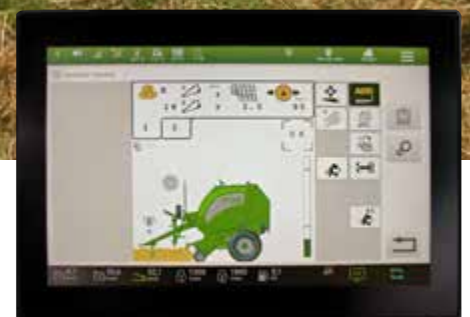
ISOBUS on a tractor terminal
