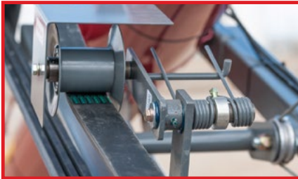
Spring Loaded Belt Idler
