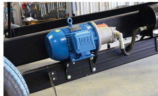
Wet Kit - used to raise and lower the conveyor if customer is wanting to run a unit on electric and doesn't have a tractor for the hydraulics to raise the conveyor
