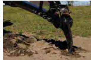
Ripper Tooth for breaking hard ground available on GX720, GX920, GX920XT
