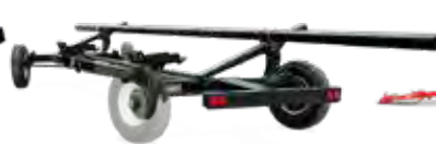
4 Wheel Steering With Rear Electric Brakes for 30' - 50' headers.
