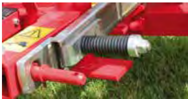
Spring loaded breakaway
