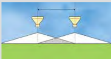
Cone shape pattern provides total overlap
