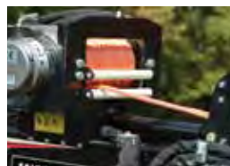
9,000 Warn Winch & 100' Synthetic Rope (RP Models)
