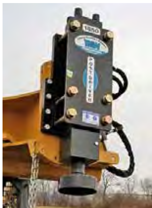
1850 Series Post Driver with Hydraulic Tilt
