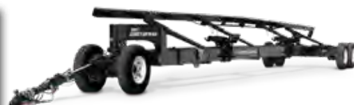
CHCTRF645 Tricycle Style Header Cart carries headers up to 45' with a tricycle-style design for stable, easy transport and maneuverability.
