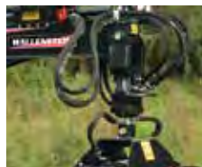
360 Hydraulic Rotator (R & PR models)
