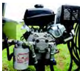
14HP commercial Kohler engine with direct mounted hydraulic pump
