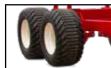
TANDEM WALKING BEAM AXLE Ensures weight is evenly distributed on the back wheels across a variety of terrain. Triangulated for increased strength the tandem axle uses two mounts reducing flex under travel.
