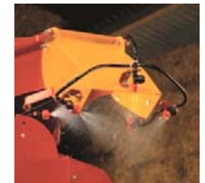
Hydro shield – dust suppression system
