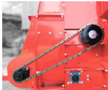
Chain drive to crossbeater for transmission of maximum power.
