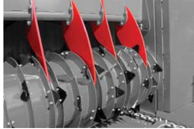
The bale restraint design works with grippers on the slats for good tumbling action, ensuring a consistently high discharge rate.
