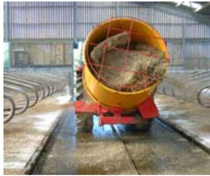
Discharging from both upper right hand and lower left hand chutes for free stall bedding. (standard on all C&B machines)
