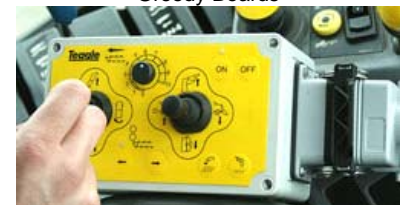
Electric Controls-Standard on all Box Type models
