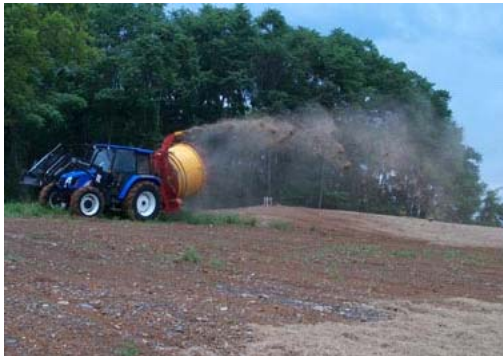
T5050 with optional Swivel Giraffe Chute operating at 1000 RPM for mulching.
