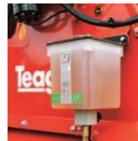
Automatic Chain Oiler (Standard on 8250)
