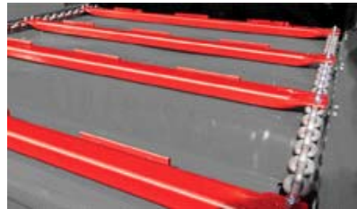
Heavy duty bed chain with slats attached by "U" bolts for easy maintenance. Grippers welded onto slats ensure good bale feed.
