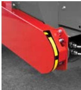
Indicator provides visual indication of bed speed.
