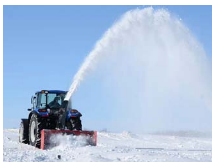
Optional hydraulic hood deflector (controlled in cab by single remote without stopping the blower).
